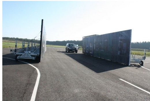
Figure 2: Brick wall Facades to replicate a reflective roadside scenario.
